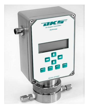
**OTT-520 PPM O2** transmitter in-line mounting equipped with 316 SS sensor housing and fittings for easy and simple installation and operation, without any external sample system. Its designed is intrinsically safe when used in conjunction with **MTL-7706** safety barrier. User selectable any range from 5 PPM to 25%. Signal output is locked on the selected range. Recovery from air to 10 PPM in under 45 minutes.
