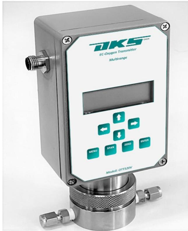
**OTT-520 PPM O<sub>2</sub>** transmitter in-line mounting equipped with 316 SS sensor housing and fittings for easy and simple installation and operation, without any external sample system. Its designed is intrinsically safe when used in conjunction with **MTL-7706** safety barrier. User selectable any range from 5 PPM to 25%. Signal output is locked on the selected range. Recovery from air to 10 PPM in under 45 minutes.
