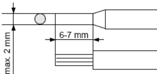
Figure 4.2. Method of cable insulation stripping and cable terminals
