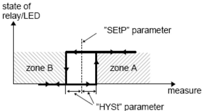
Figure 6.4. One threshold control of the relay/LED outputs
