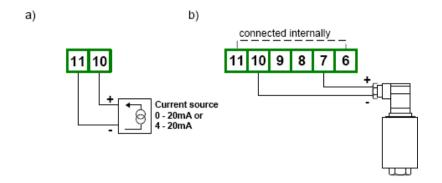
Figure 4.11. Connections of 2-wire sensor:
