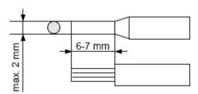
Figure 4.2. Mehtod of cable insulation replacing and cable terminals
