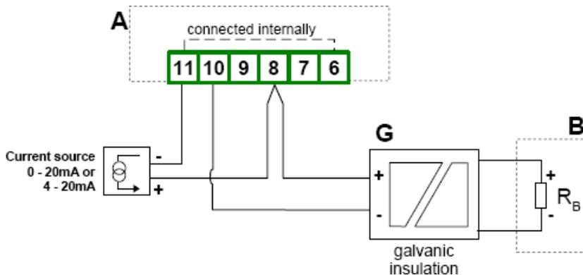
Figure 4.12. Serial connection of active 2-wire sensor with **PD96** unit and other current measurement device (e.g. PLC controller)
