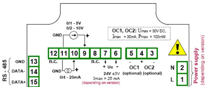
Figure 4.4. Terminals description (OC-type outputs)
