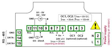
Figure 4.4. Terminals description (OC- type outputs)
