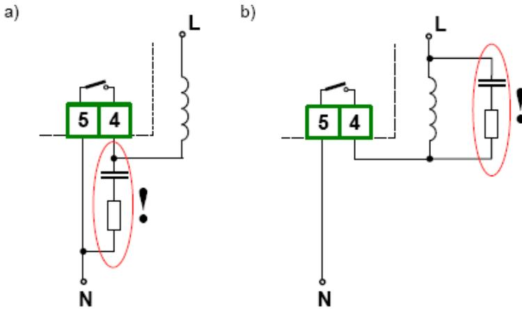
Figure 4.9. Examples of suppression circuit connection:
