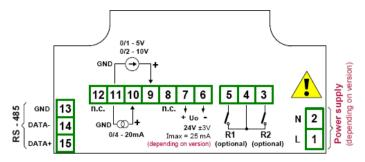
Figure 4.3. Terminals description (relay outputs)
