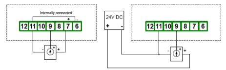
Figure 4.7. Connection of voltage converters
