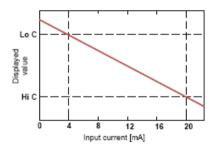
Figure 10.1.Normal ("Lo C" < 2Hi C) and inverted ("Lo C" > "Hi C) characteristic
