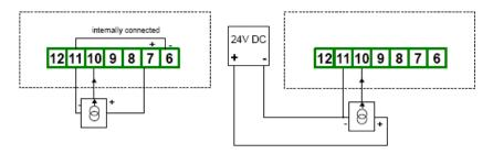
Figure 4.6. Connection of 3-wire current converters
