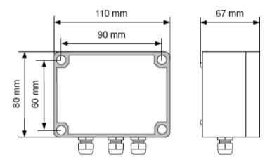
Figure 4.1. Device and assembly dimensions
