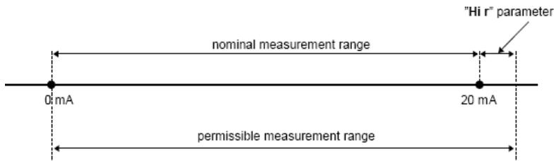
Figure 3.2. Definitions of measurement ranges in mode 0 ÷ 20mA
