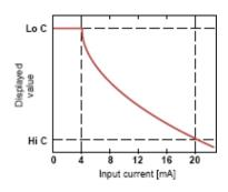
Figure. 10.3 Normal ("Lo C" < "Hi C) and inverted ("Lo C" > "Hi C) characteristic
