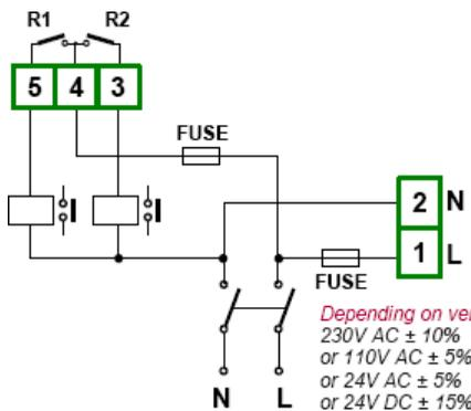
Figure 4.8. Connection of power supply and relays
