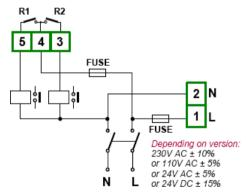
Figure 4.8. Connection of power supply and relays
