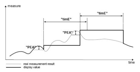
Figure 6.3. Process of peaks detection
