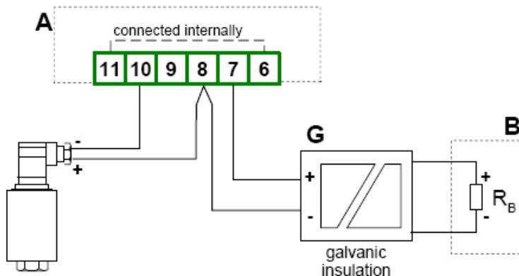
Figure 4.13. Serial connection of passive 2-wire sensor with **PD96** unit and other current measurement device (e.g. PLC controller).
