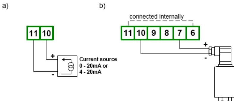
Figure 4.11. Connections of 2-wire sensor:
