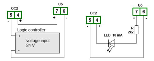
Figure 4.10. Example of OC-type outputs connection
