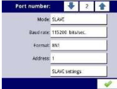
Fig. 7.150. Configuration parameters for **SLAVE** mode
