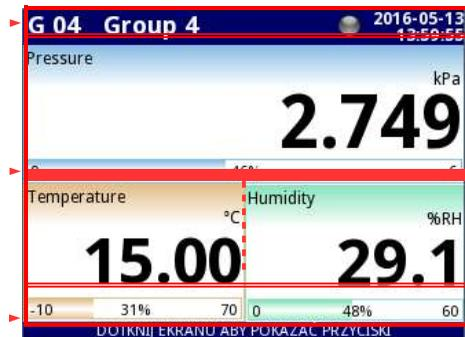
Fig. 6.4. Typical view of the **CONTROLLER/DATA RECORDER** main page, after touching the display
